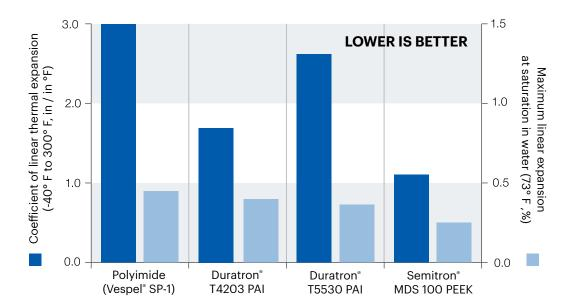
Semitron® MDS 100 modified Polyetheretherketone PEEK shapes offer a remarkable combination of strength, stiffness, and stability. This grade in particular was developed for use in controlled application environments where a high level of precision is required. Due to this, Semitron® MDS 100 components are often used as test sockets, nests, and fixtures in test and package equipment throughout the semiconductor and electronics industry.
