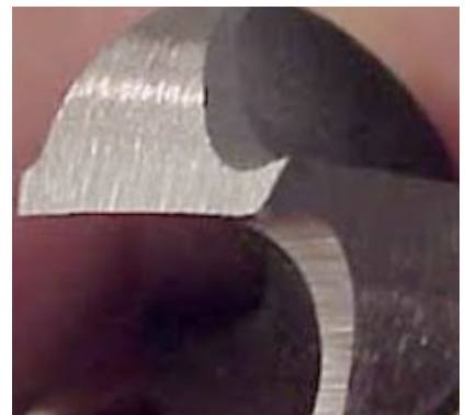
Thinning of web is recommended on larger drills
