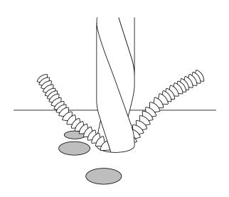
1/2" diameter) using 600 to 1,000 rpm and a positive feed of 0.005" to 0.015" per revolution.
