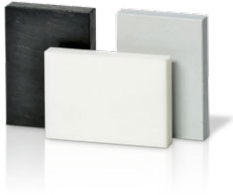
**Tech Notes:** Since Ertalyte® tends to be rather notch and impact sensitive, all “internal” corners should be radiused [R > 1 mm] and to avoid chipping the edges during turning, boring or milling, chamfered edges are advantageous, providing a smoother transition between the cutting tool and the plastics work.
