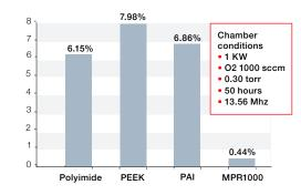
Semitron<sup>®</sup> MPR1000 has less than 0.5% erosion in 1KW O2, 13x better than Pl
